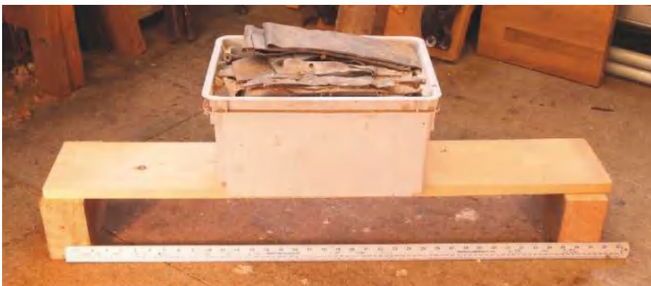
▲ Pic.2 Home-made bending test. Load a sample with a heavy weight and see how far apart the supports need to be. But if you don't want your shelves to bend over the years, then allow a healthy safety factor!
